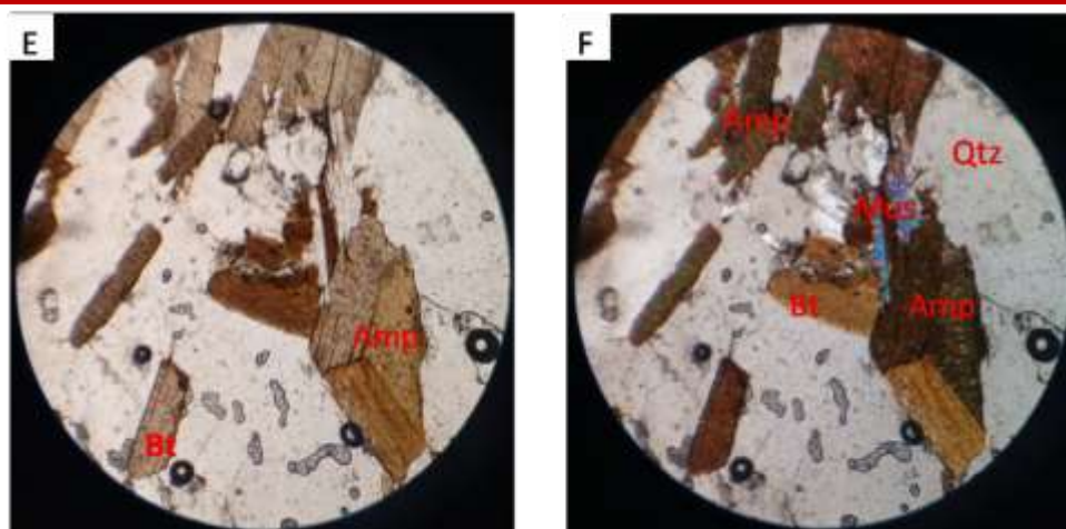
Plate V: Photograph of Field and Hand Sample of Schist (A and B) and Photomicrograph under both PPL and XPL (C, D, E and F). Qtz: Quartz, Bt: Biotite, Mus: Muscovite, Opq: Opaque, Sil: Silimanite. (Mag. X40; E, F=X100)
